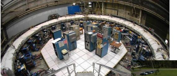
52-foot-wide electromagnetic ring for catching muons
