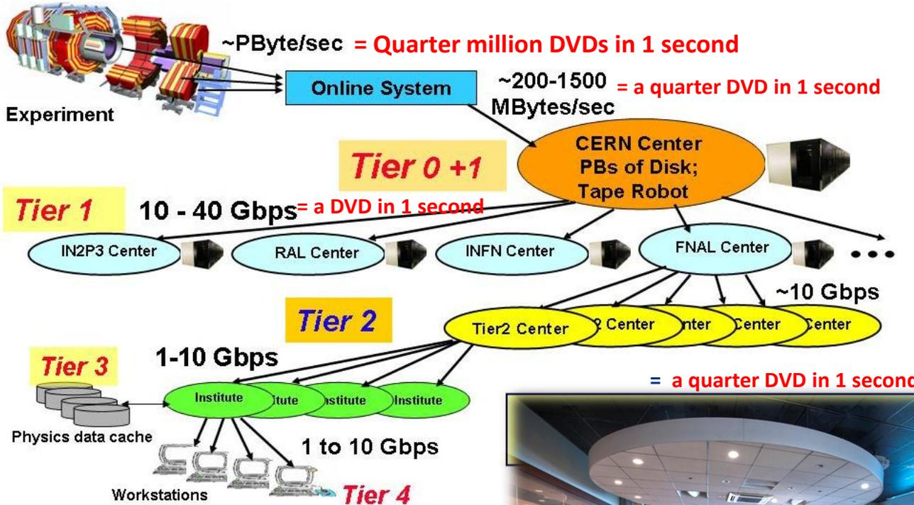
The distributed computing system for LHC distributes hundreds of Terabytes a day outward from CERN to the 11 distributed Tier-1 sites (one at Fermilab) & then 25 University Tier-2 and access to more than 100 smaller Tier-3 centers.
