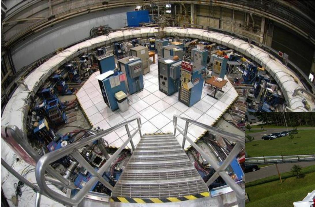
52-foot-wide electromagnetic ring for catching muons
